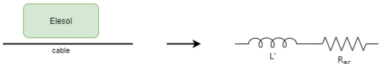
Figure 5: Circuit equivalent of Elesol plate.
