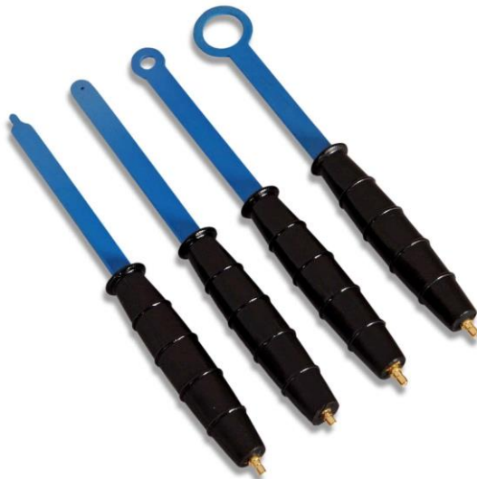
Figure 11: Near Field prob for conducted and emitted emission test.
